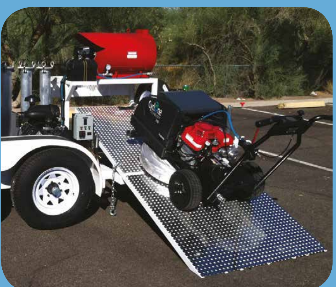
Pivoting ramp allows winch easy loading and unloading of the CY210 walk-behind.
