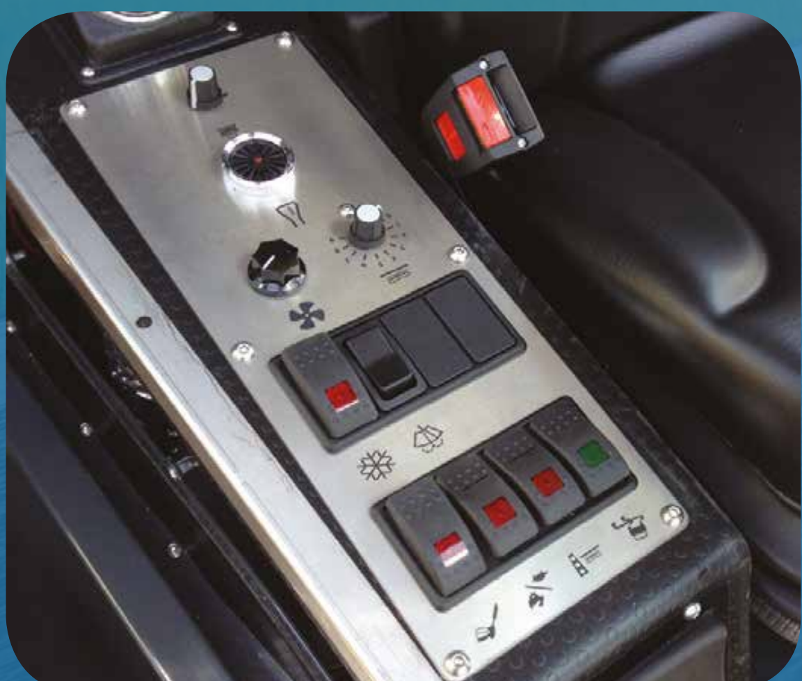
Infinitely variable water pressure and cleaning speed is easily controlled from the operator's seat, for a full clean on various surfaces.
