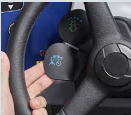
Intermittent SmartFlow™ lever integrated into steering wheel: Reduces water flow on the deck, preventing splashes during turns, lowering consumption and ensuring perfect drying performance
